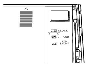
Clock speed-Slide the CLOCK switch to the left to select a CPU clock speed of 8 MHz. Leave the switch in the right position to select a CPU clock speed of 12 MHz.
